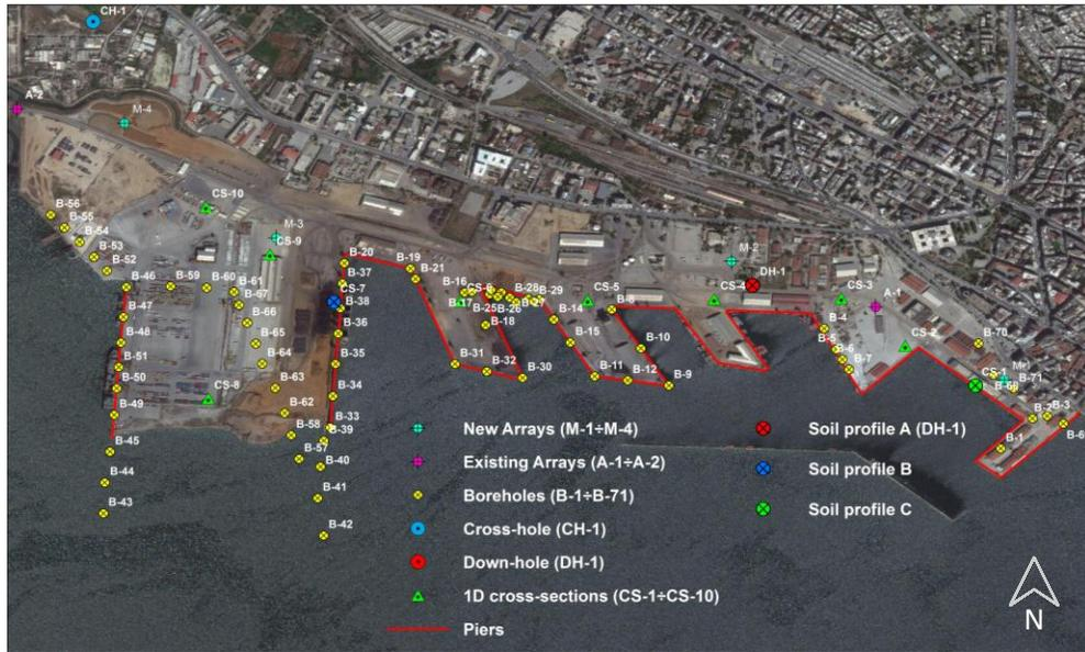
Fig. 3 – Location of geotechnical and geophysical field measurements in Thessaloniki’s port area.
